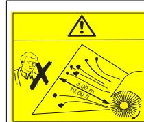
Hazard caused by ejected parts with moving roller brush. Keep a safety distance of 3 m towards the front and the side
